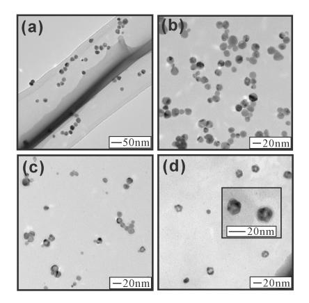
Fig. 1. TEM images Ag NPs (a), and Ag@Au NPs with atomic feeding ratio of: 5 % Au (b), 15 % Au (c), and 25 % Au (d).
