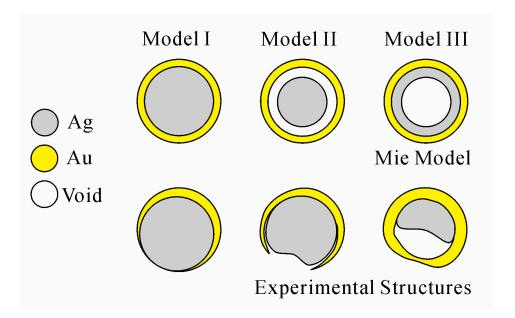
**Fig. 4.** The Mie Model structures of Ag@Au NPs used with the Mie solution along with the corresponding experimental structures.
