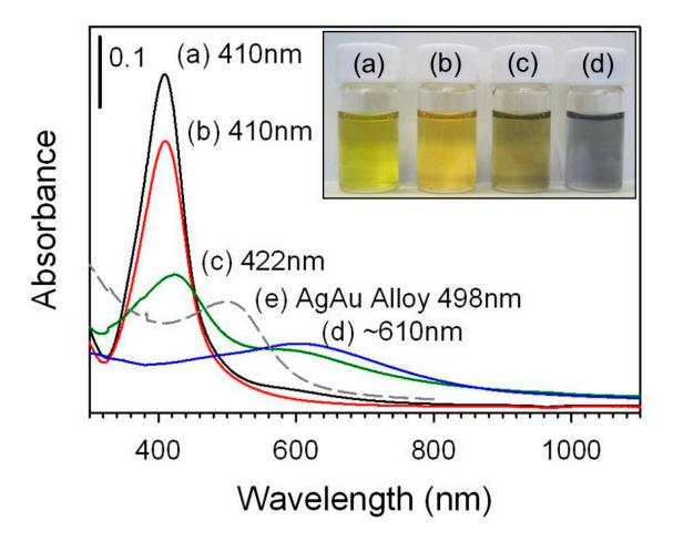
**Fig. 2.** UV-vis spectra for Ag and Ag@Au NPs prepared with increasing Au content, as-synthesized Ag NPs (a), 5 % Au atomic feeding ratio (b), 15 % Au atomic feeding ratio (c), 25 % Au atomic feeding ratio (d), and a Ag-Au NP alloy (e). The inset shows the photographs of the Ag and Ag@Au NPs.
