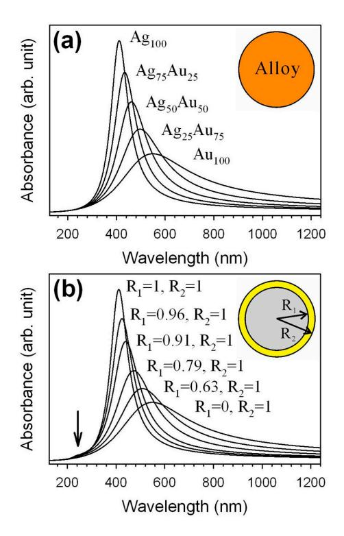
**Fig. 5.** UV-vis spectra calculated using the Mie solution for alloy Ag-Au NPs (a), and for Ag@Au NPs with the Model I structure (b).
