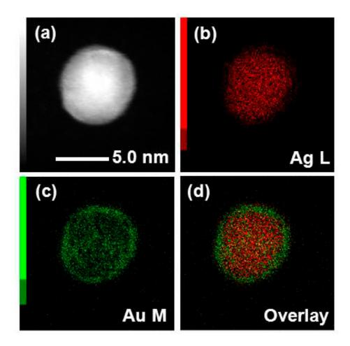
**Fig. 3.** High-angle annular dark-field STEM image (a) and EDS mapping of Ag (b) and Au (c) in a single NP. The overlay image (d) shows the relative location of Ag and Au in a single NP. The scale bar applies to all images.
