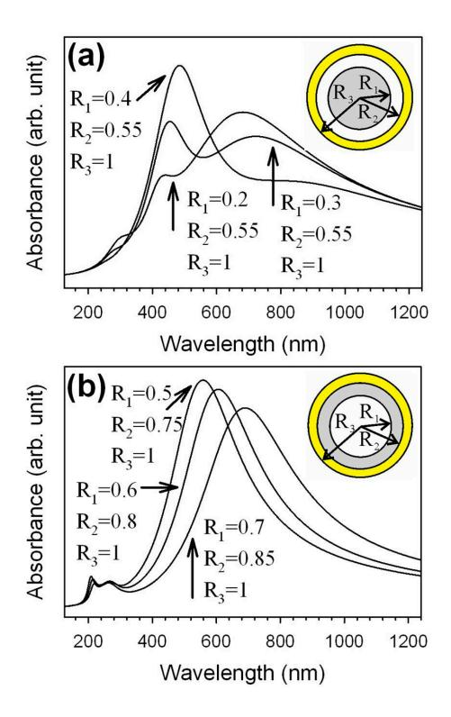
**Fig. 6.** UV-vis spectra calculated using the Mie solution for Ag@Au NPs using Model II (a), and for Ag@Au NPs using Model III (b).
