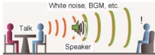
Fig. 1 – Speech privacy protection by power masking with white noise, pink noise, BGM, etc.
