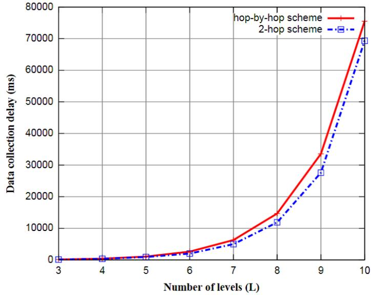
Figure 3.13: Binary tree network – expected decrease in data collection delay with 2-hop scheme over hop-by-hop scheme
