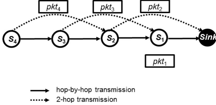
Figure 3.11: A chain topology network consisting of 4 sensors
