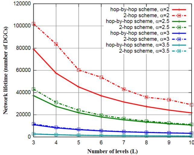
Figure 3.3: Chain network – network lifetime with hop-by-hop scheme and expected network lifetime increase with 2-hop scheme for different path loss exponents
