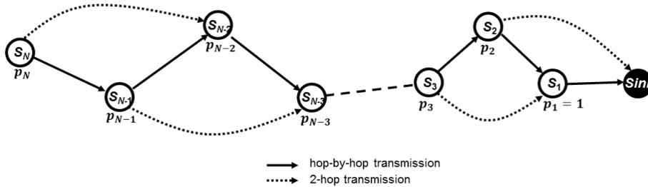
Figure 3.1: A chain topology network of  $N$  sensors
