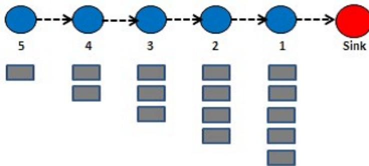
Figure 1.2: Unbalanced energy consumption caused by multi-hop transmission
