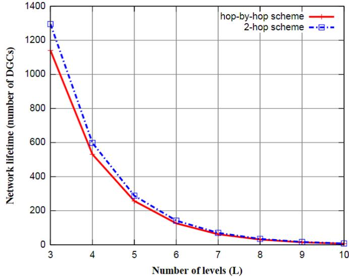
Figure 3.6: Binary tree network – expected network lifetime increase with 2-hop scheme ( $\alpha = 3.5$ )
