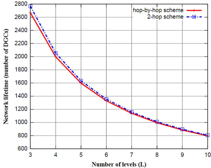
Figure 3.2: Chain network - network lifetime with 2-hop scheme and hop-by-hop scheme ( $\alpha = 3.5$ )
