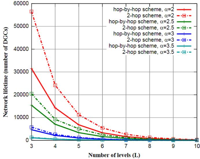
Figure 3.7: Binary tree network – network lifetime with hop-by-hop scheme and expected network lifetime with 2-hop scheme for different path loss exponents
