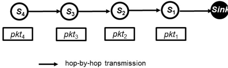
Figure 3.10: A chain topology network consisting of 4 sensors
