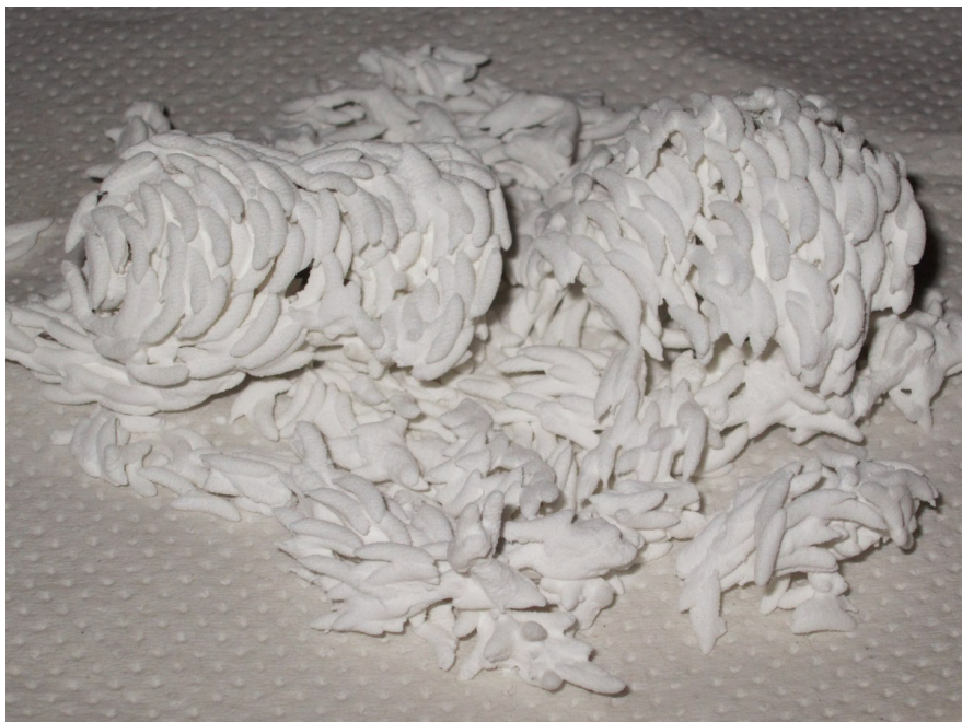
Figure 4.19: Broken printed aggregate.
