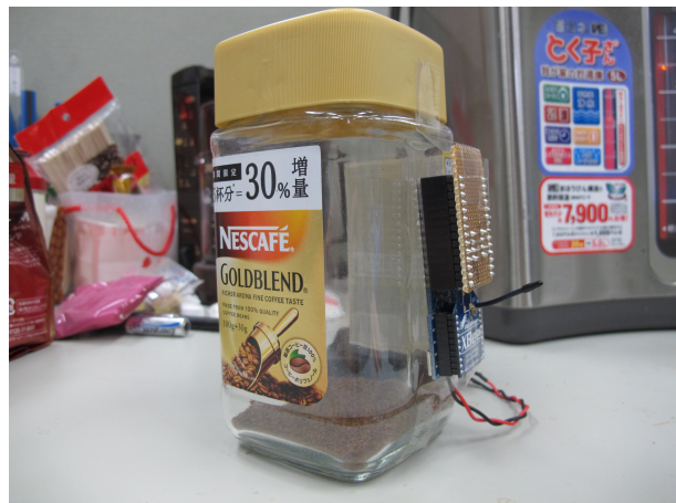
(b) The “Coffee Container” with gyro sensor
