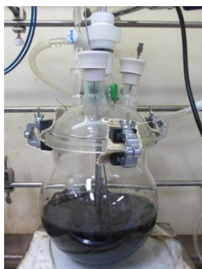
Figure 5.1. Photograph of the reactor after 1 hour of reaction with the black dispersion of the resulting NPs in di-phenylether. The reaction solution volume is of about 1070 mL.
