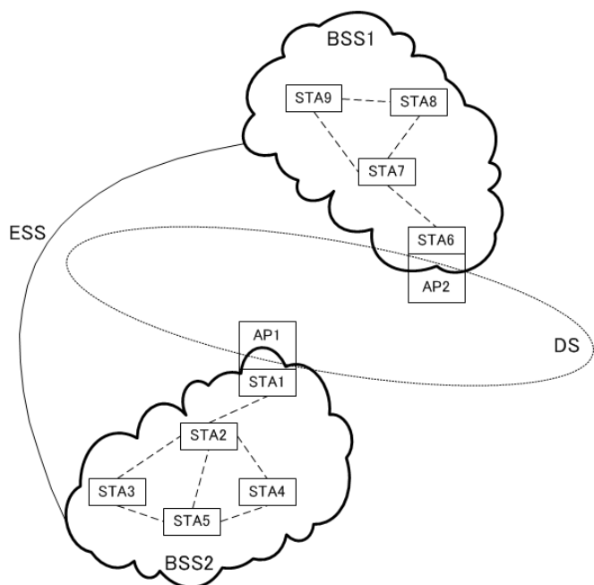
Fig.2 Example device consisting of mesh STA and AP STA to connect an MBSS and an infrastructure BSS
