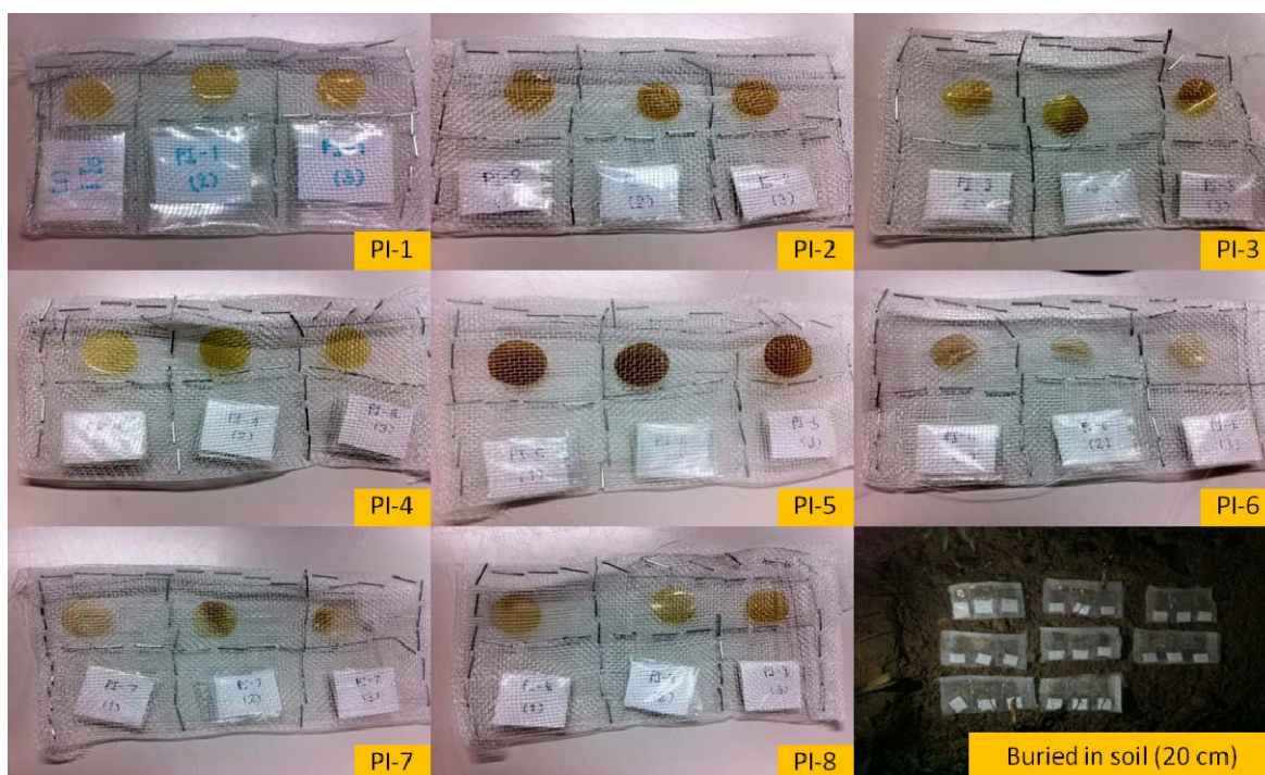
Figure 4.6 Physical appearances of PI films before burring in soil for degradation behavior in an environment under light, rainwater, moisture and bacteria.
