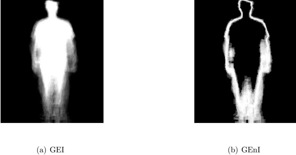
Figure 3.1: Gait representation using binary images
