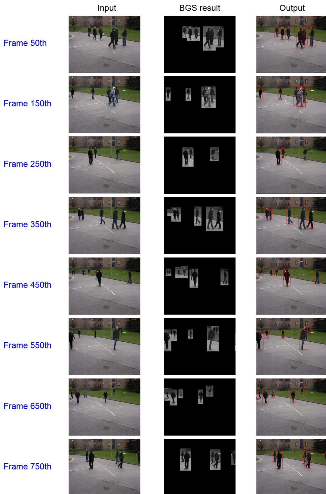
Figure 6.10: The detection result on the S2.L1.008 sequence. Detected pedestrians are marked by red bounding boxes.
