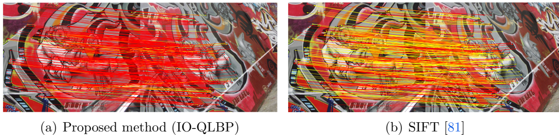
Figure 1.8: Two matching results provided by the proposed IO-QLBP and the baseline SIFT[81] descriptors. Red lines indicate correspondences that are correctly identified, whereas yellow lines describe correspondences that the descriptor fails to match.
