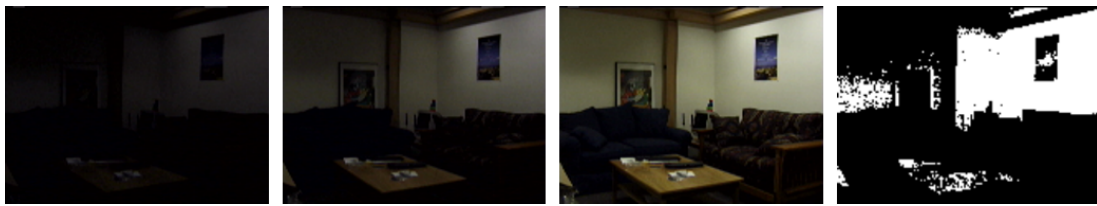
(a) Gradual illumination change. The first three images presents an indoor scene with increasing illumination. The last image shows the background image created by the MOG [124]
