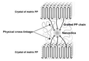
Figure 1. Structure of physical cross-linkage
