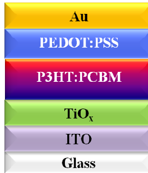
Fig. 3.7: Structure of inverted BHJ device
