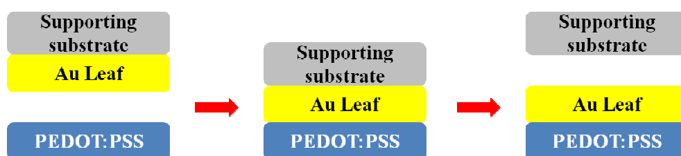
Fig. 4.1: Condition when the W between Au/PEDOT:PSS higher than the W between Au/supporting substrate.
