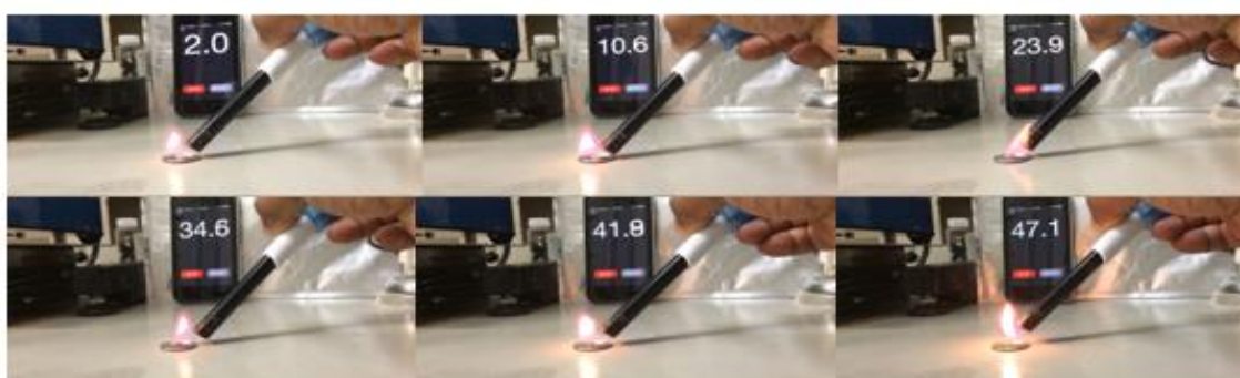
Time-sequenced flammability studies of Hybrid B
