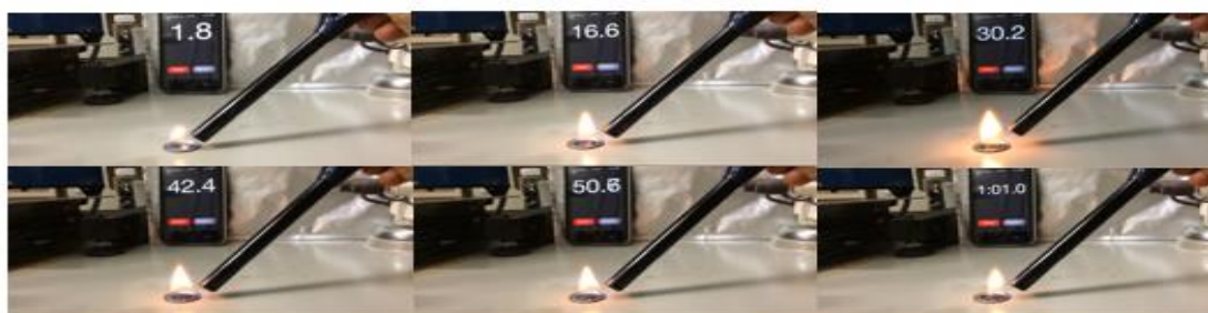
Time-sequenced flammability studies of Hybrid H
