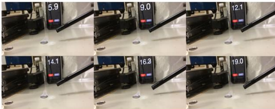
Figure 4.19 Flammability studies of 1MLiPF 6 (1:1 EC-DEC) solution
