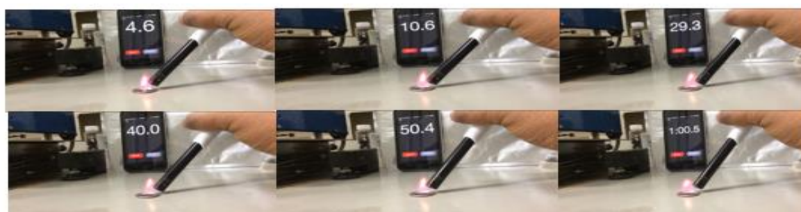
Time-sequenced flammability studies of Hybrid C
