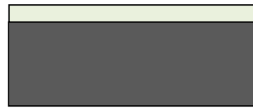
The cross-sectional view of c-Si passivated by \text{SiN}_x film. Sample size is 2 \times 2 \text{ cm}^2
