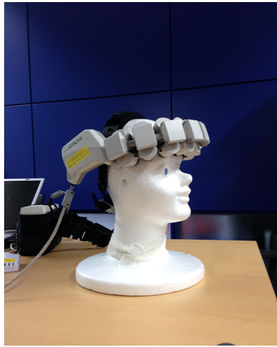
Figure 4.1: Full mobility 22-channel fNIRS array (courtesy Fujinami Laboratory, JAIST School of Knowledge Science)
