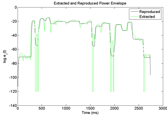
Figure 6: Reproducing power envelope using 2nd-order critically damped model and the extracted power envelope from original speech
