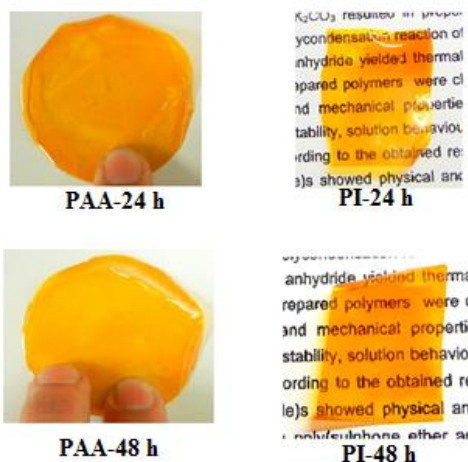
Figure 3.15 PAA and PI films of polymers prepared from DAS and mixed dianhydrides (BTDA and DSDA).
