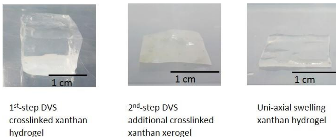
Figure 3.10 Xanthan gum hydrogels prepared by two-step DVS cross-linking.
