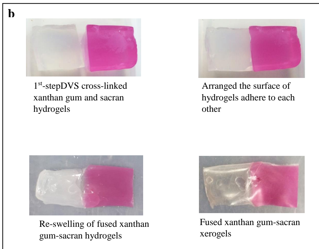
Figure 3.11 Representative fused DVS cross-linked LC hydrogels. (a) sacran-sacran hydrogels with no-color and pink color sacran. (b) sacran-xanthan gum hydrogels, no color xanthan gum and pink color sacran.
