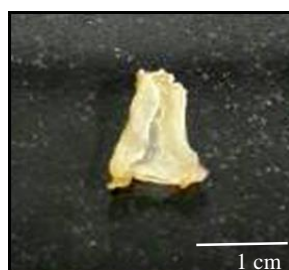
Figure 3.5 Xerogel formed by dehydration with ethanol and vacuum dried.
