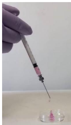
Figure 19 (b) Illustration of nanocomposite N_6P(65)_{1.5} that can be injected through 22G needle
