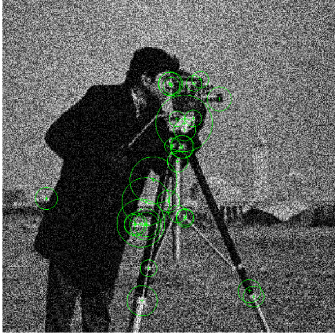
Figure 4.11: Surf features of noised cameraman image.
