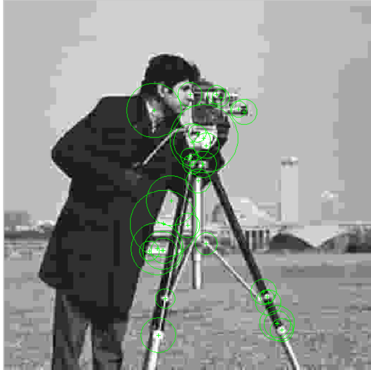
Figure 4.9: Surf features of compressed cameraman: JPEG 5%.
