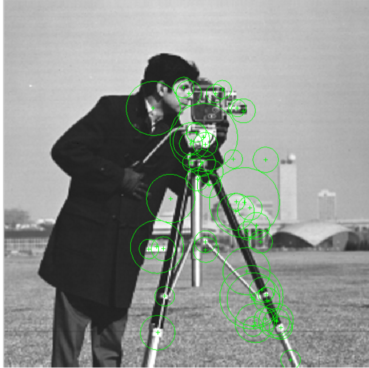
Figure 4.8: Surf features of original grayscale cameraman image.
