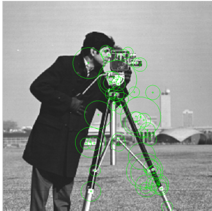
Figure 4.8: Surf features of original grayscale cameraman image.
