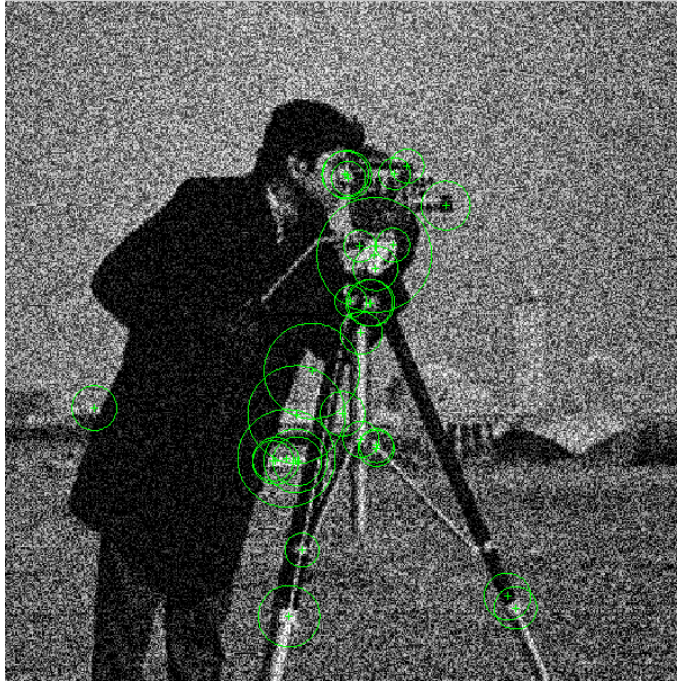
Figure 4.11: Surf features of noised cameraman image.
