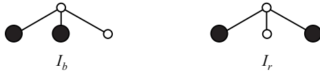
Fig. 2. A yes-instance for ISRECONF under the TJ rule, which is a no-instance for the SLIDING TOKEN problem.
