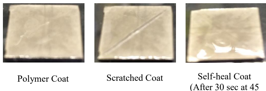
Figure 3.18: Visual Observation of Self-healing Property of 2.
