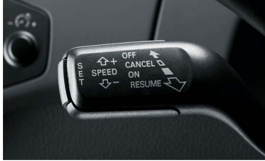
Fig. 1. Function buttons on the control lever of cruise control system. (The figure is from the home page of Audi)
