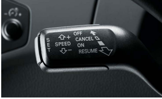
Fig. 1. Function buttons on the control lever of a cruise control system. (The figure is from the home page of Audi.)
