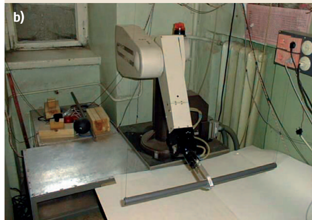
Figure 44.10: A web-based teleoperation system that allows a robot to capture a fast-moving rod [27] (a) User interface and (b) system setup
