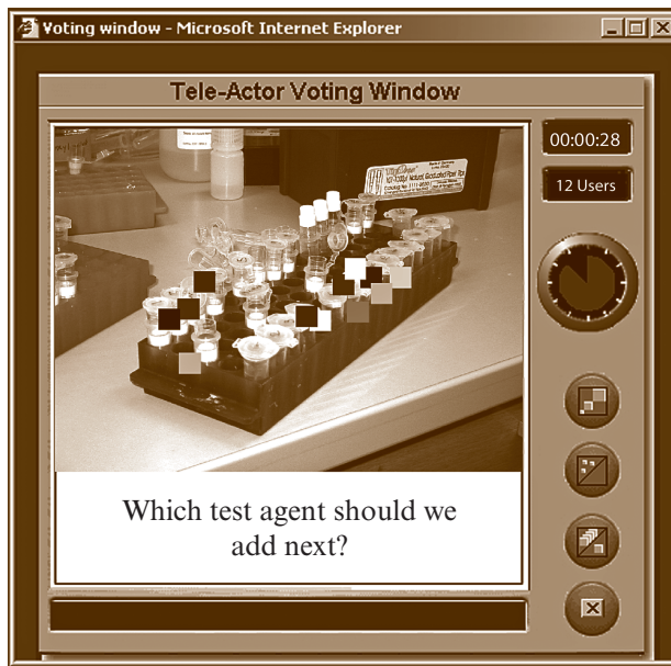
Figure 44.11: Spatial dynamic voting interface for the Tele-Actor system [52]: the spatial dynamic voting (SDV) interface as viewed by each user. In the remote environment, the Tele-Actor takes images with a digital camera, which are transmitted over the network and displayed to all participants with a relevant question. With a mouse click, each user places a color-coded marker (a votel or voting element) on the image. Users view the position of all votels and can change their votel positions based on the group’s response. Votel positions are then processed to identify a consensus region in the voting image that is sent back to the Tele-Actor. In this manner, the group collaborates to guide the actions of the Tele-Actor
