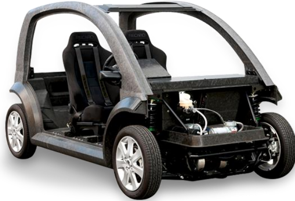
Figure 1: Car made by Teijin Japan from CFRP material. Pic courtesy: Teijin website.
