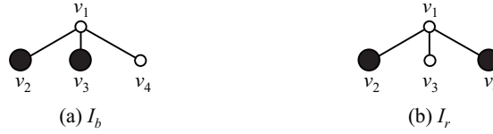
Figure 2: Two distinct independent sets I_b and I_r of the same star. This is a yes-instance for ISRECONF under the TJ rule, but is a no-instance for the SLIDING TOKEN problem.
