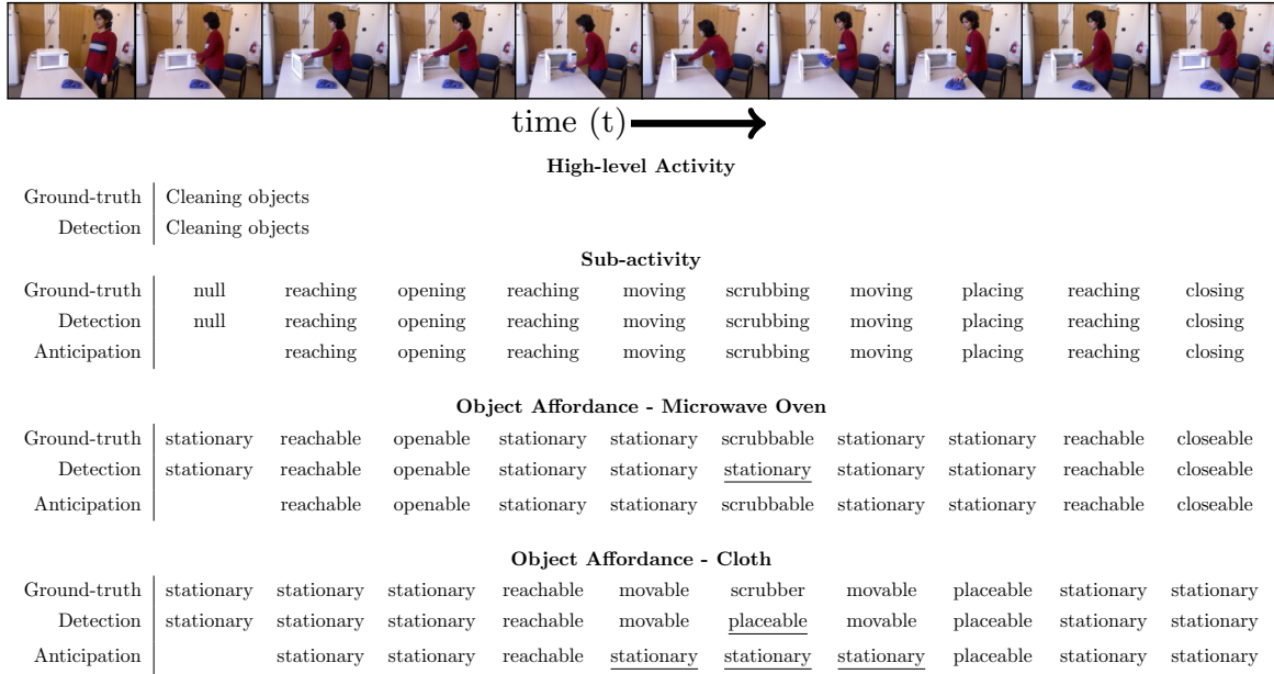
Figure 4.7: An example result on cleaning activity on CAD-120. This figure shows the success and failure cases (underlined) of detection and anticipation results of S-RNN.
