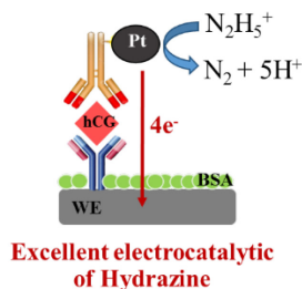
Figure 4. Schematic illustration of the electrocatalysis of hydrazine by PtNPs
