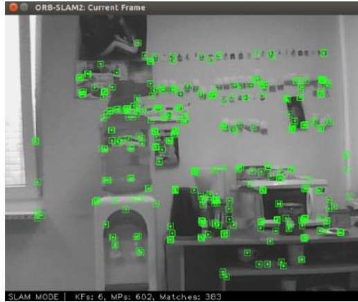
(a) Feature extraction for ORB-SLAM [12]
