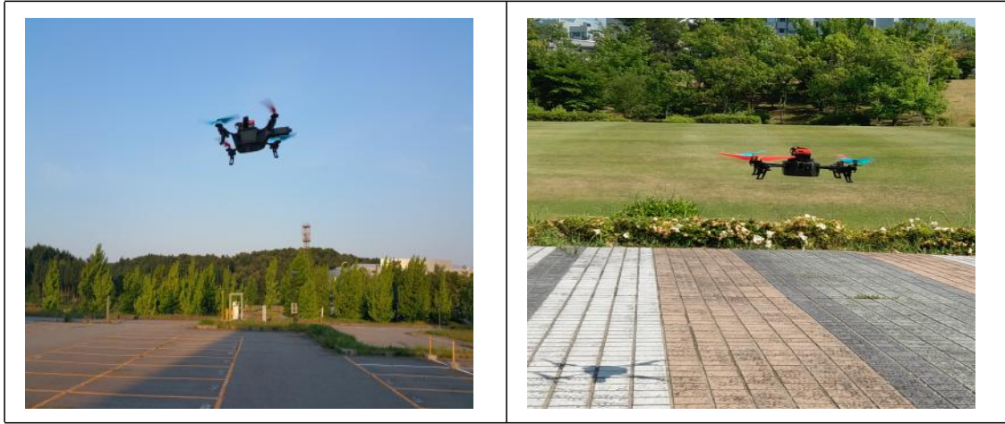
Figure 5.13: ArDrone 2.0 with GPS used for outdoor experiments in parking lot and public park.
