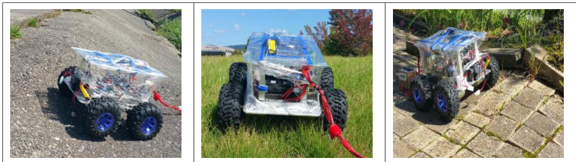
Figure 5.12: Rusti V2.0 with all-terrain wheels and external 3-axis accelerometer sensor for outdoor field experiments carried out on asphalt, grass and tiles.
