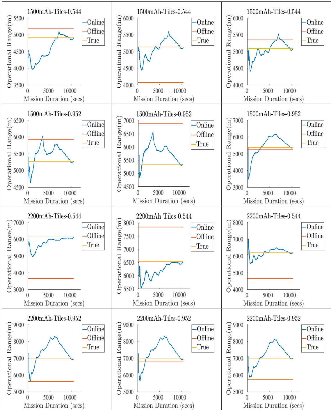
Figure 5.21: Rusti's operational range estimation for tiles. Rows 1 – 2 represent experiments performed using 11.1V@1500mAh battery @80rpm followed by @140rpm. Rows 3 – 4 represents the similar pattern for 11.1V@2200mAh battery respectively.
