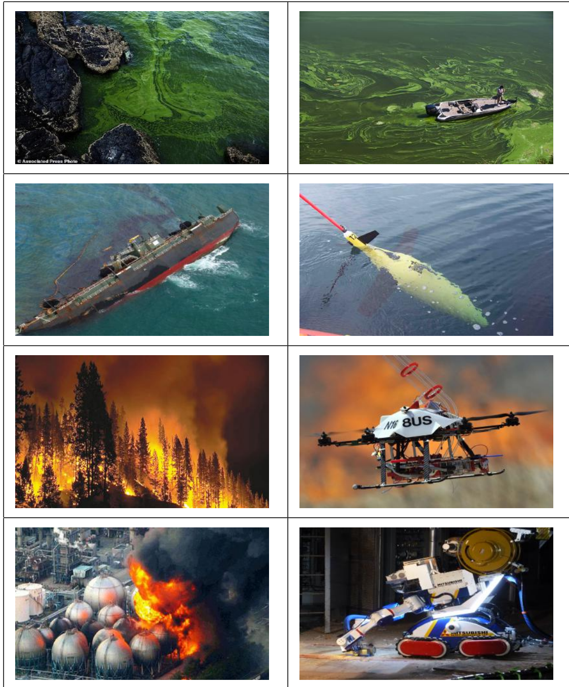
Figure 1.1: Environmental Monitoring Scenarios. The top row shows algal bloom [21] on the left which can be monitored using surface vehicles as shown on the right [22]. The second row shows the oil spill off the coast of Gulf of Mexico [23] which can be monitored using underwater gliders [24] and the third row shows forest fires [25] which can be monitored using multi-rotor UAVs [26]. The bottom row shows the fukushima daichii nuclear disaster [27] and one of the robots that were used to assess the damage [28].
