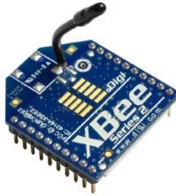
Figure 2.11: XBee ZB ZigBee Mesh Module 2.4GHz 2mW with Wire Antenna for short-range wireless communication [22].
