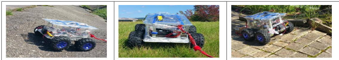
Figure 2.12: Rusti V2.0 with all-terrain wheels and external 3-axis accelerometer sensor for outdoor field experiments carried out on asphalt, grass and tiles.
