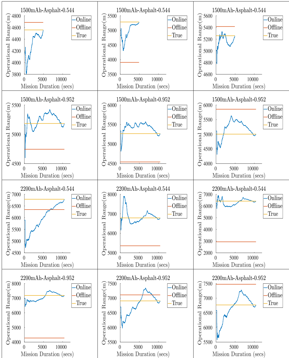
Figure 5.20: Rusti's operational range estimation for asphalt. Rows 1 – 2 represent experiments performed using 11.1V@1500mAh battery @80rpm followed by @140rpm. Rows 3 – 4 represents the similar pattern for 11.1V@2200mAh battery respectively.
