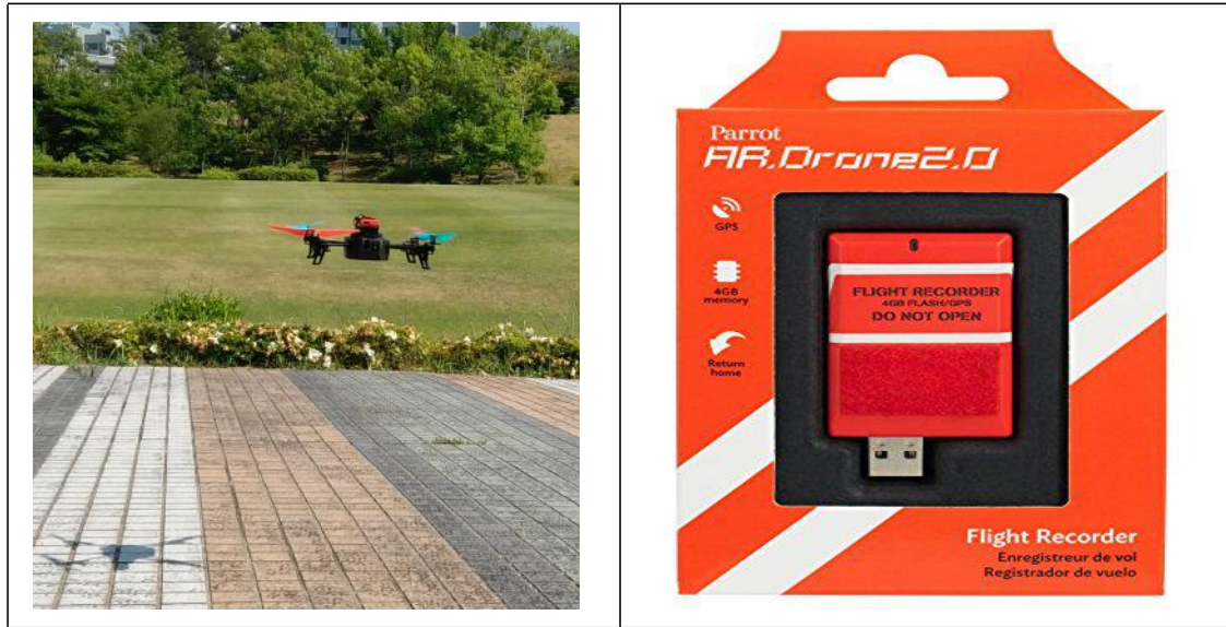
Figure 2.8: ArDrone 2.0 with GPS flight recorder [21] used for outdoor experiments.
