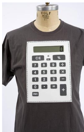
Figure 2.24: Pressure sensors based calculator embedded into T-shirt
