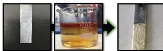
Fig. 3 Illustration of growth of MOF-5 (IL) films
