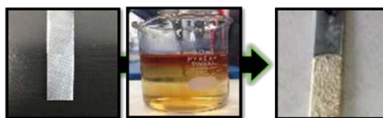
Fig. 3 Illustration of growth of MOF-5 (IL) films on zinc surface during electrochemical synthesis.
