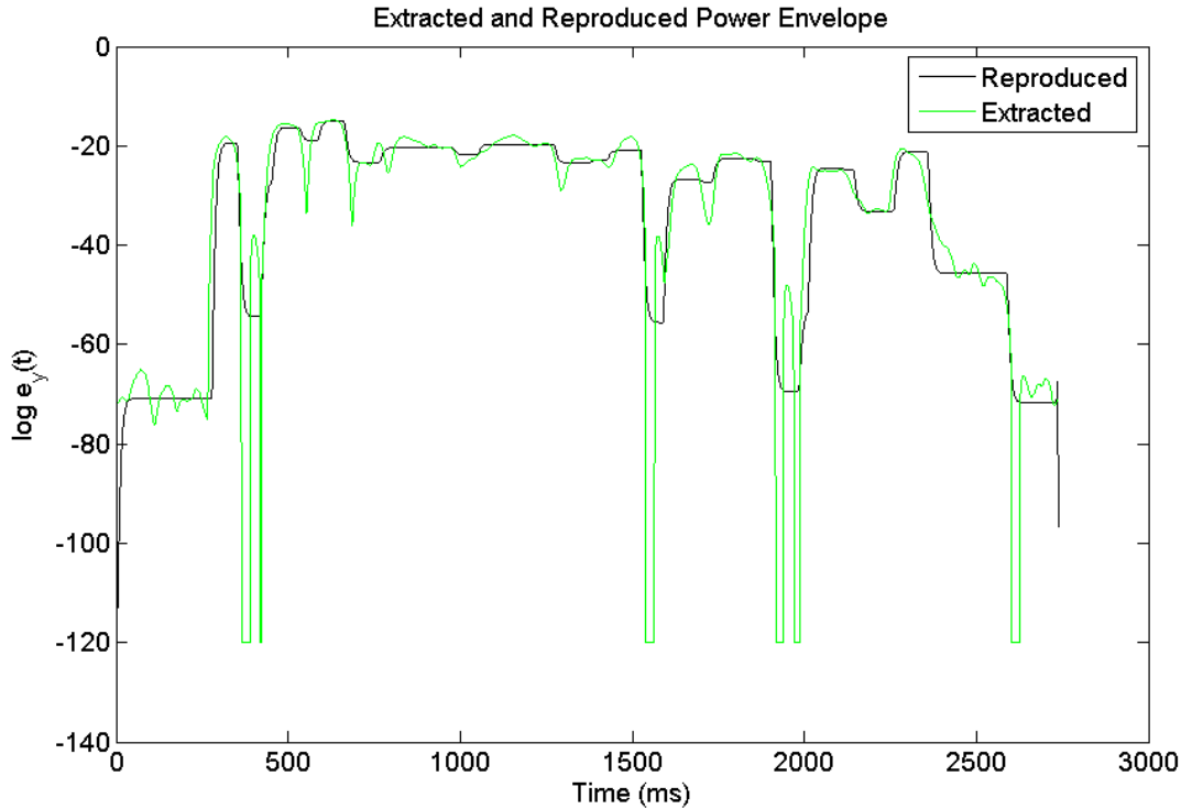
Figure 5.14: Reproducing power envelope using 2nd-order critically damped model and the extracted power envelope from original speech
