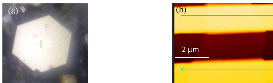
Figure 1. (a) Optical image of a \text{Mo}_{0.97}\text{Nb}_{0.03}\text{S}_2 flake and (b) AFM image of ultrathin layer.
