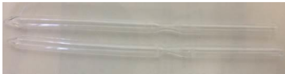
Figure 2.1 Quartz ampoules used for the CVT growth of single crystals.
