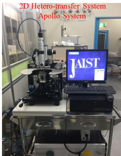
Figure 3.8 The Apollo System for transferring ultrathin layer onto electrodes.
