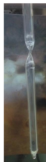
Figure 2.3 Narrow-necked part of ampoule.
