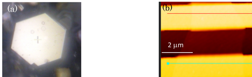
Figure 1. (a) Optical image of a Mo 0.97 Nb 0.03 S 2 flake and (b) AFM image of ultrathin
