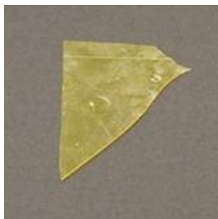
Figure 2.5. Photograph of a blend film of PMMA/LiNO 3 ([Li]/[C=O] ratio of 0.07).
