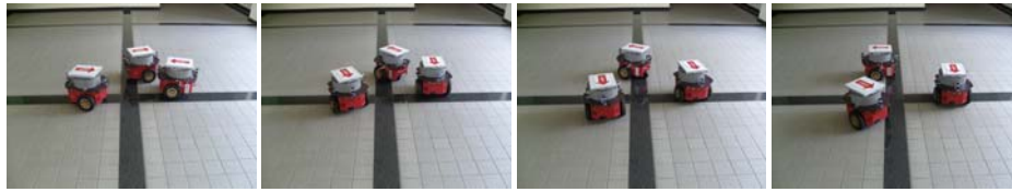
Fig. 11 Experimental results for self-configuration from a random configuration of 3 robots
