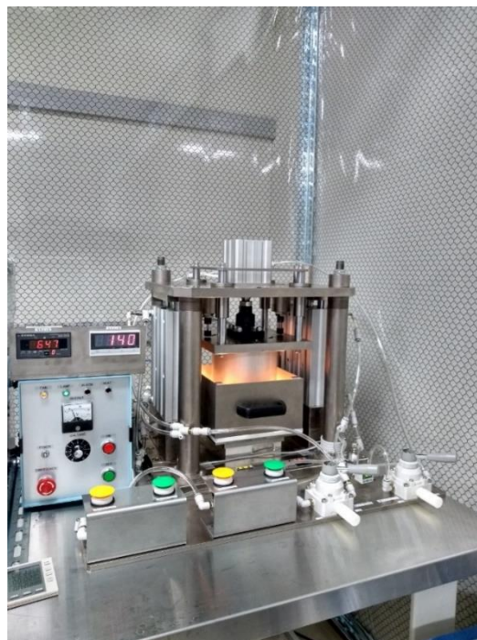
Fig. 3-5: n-RP machine during imprinting.
