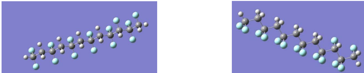
Figure 6.1. Chemical structure of (a) \alpha -phase P(VDF-TrFE) (b) \beta -phase P(VDF-TrFE)
