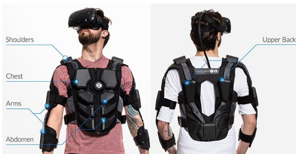
Figure 1.1 Hardlight suit invented by Hardlight VR
