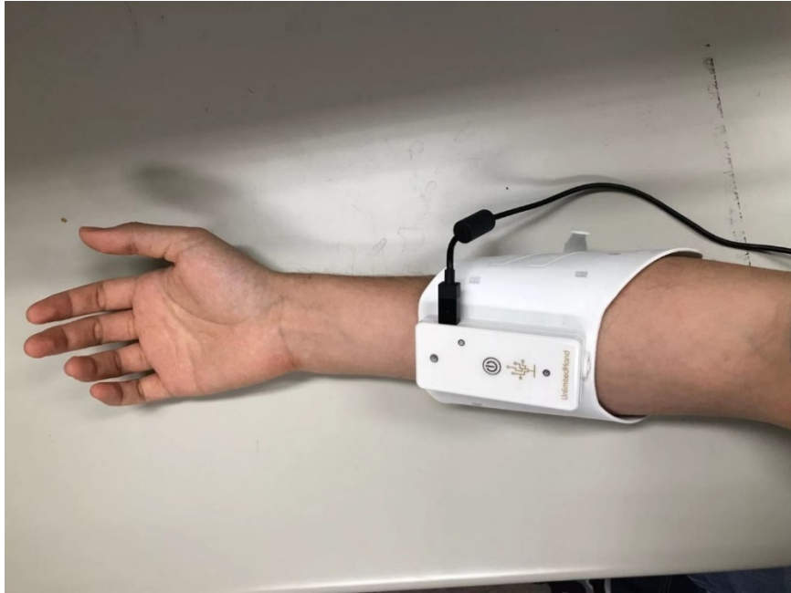
Figure 2.4 How to wear the UnlimitedHand.
