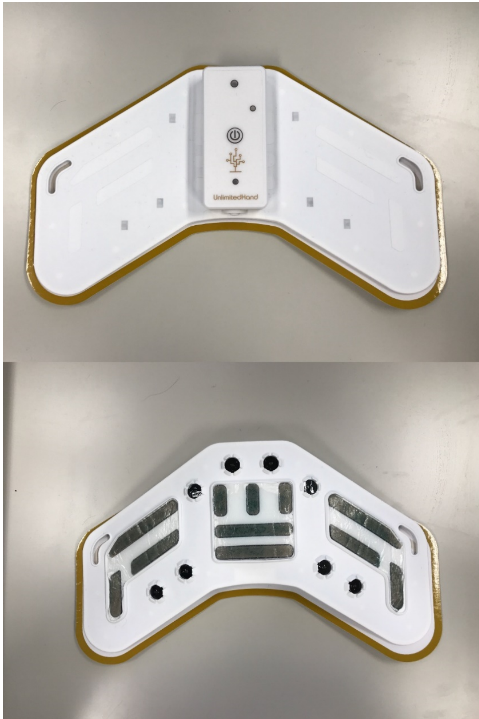
Figure 2.3 The outside and inside of the UnlimitedHand
