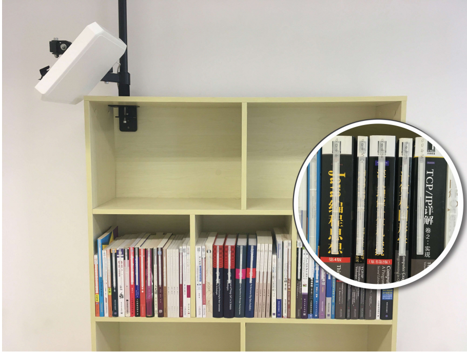
Figure 5-6: The white antenna is placed at a 45^\circ angle to the ground to ensure it can cover as much region as possible, because of its fan-shaped radiation regions.
