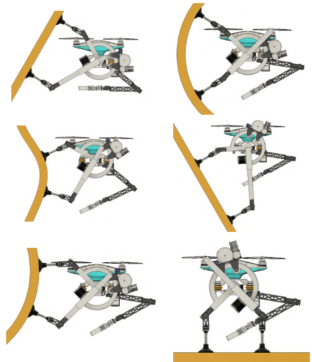
Fig. 5: Some examples of landing on arbitrarily shaped surfaces. Only core stander setups are illustrated. This mechanical design is flexible to any shape of the surface thanks to its swivel arms. Swivel arm and vacuum suction cups are adjustable according to the shape of the surface to be landed.
