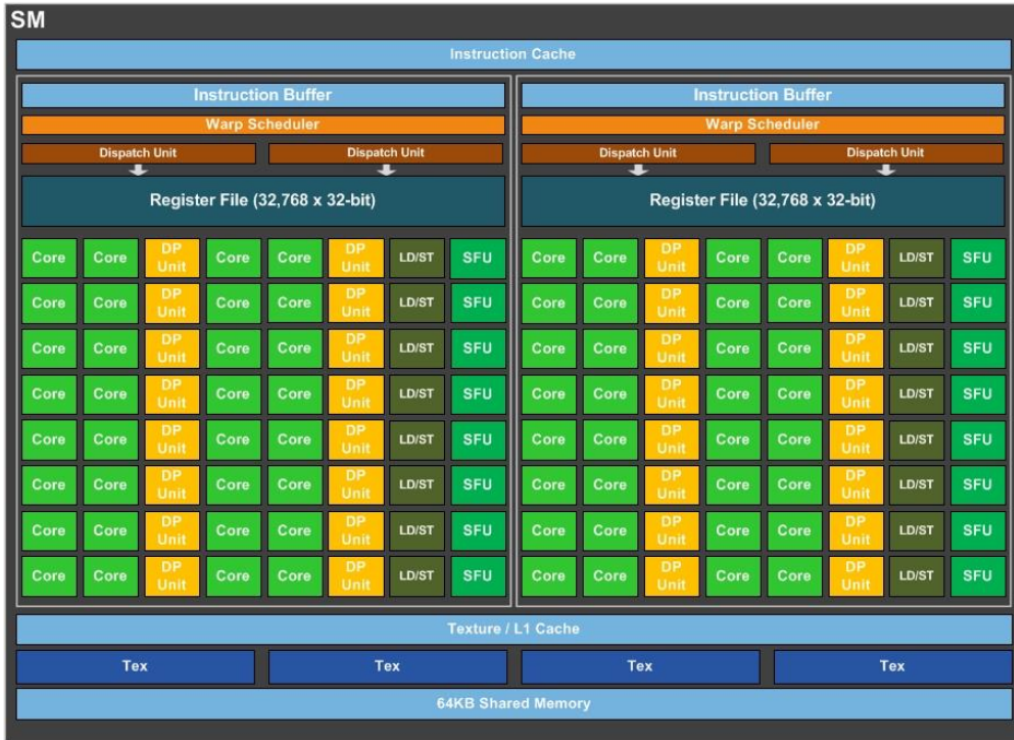
Figure 2.3: Pascal GP100 SM unit architecture (quoted from [1])
