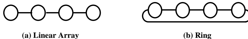
Figure 2.3: A four-node linear array and ring network
