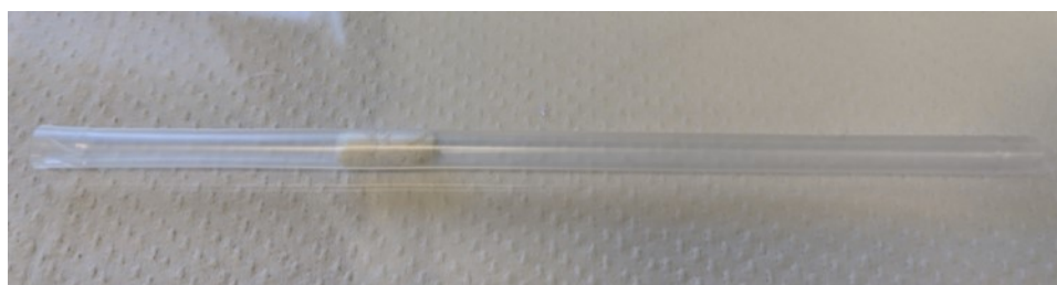
Figure 5.2: Plastic straw with sample sandwiched between two pieces of Kimwipe for magnetic measurements.
