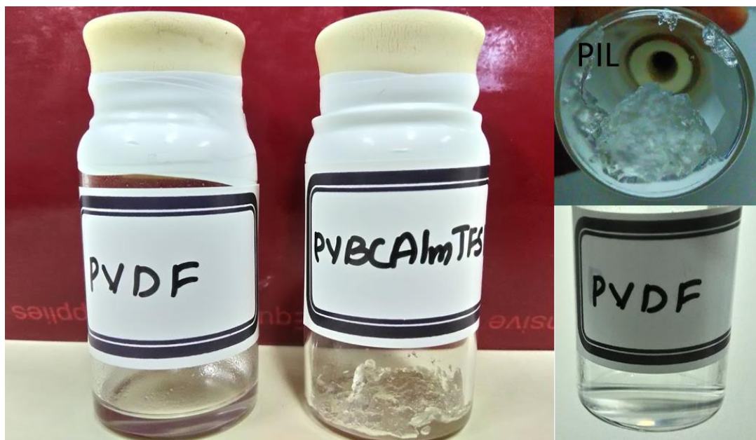
Figure 2.25 Photographs of wettability test to evaluate the interaction of the binders with electrolytes.
