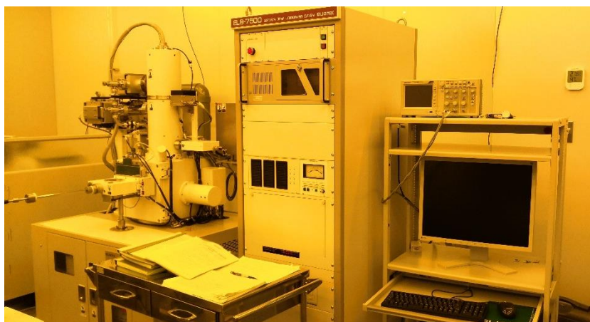
Figure 2.4 Photograph of Electron Beam Lithography machine.
