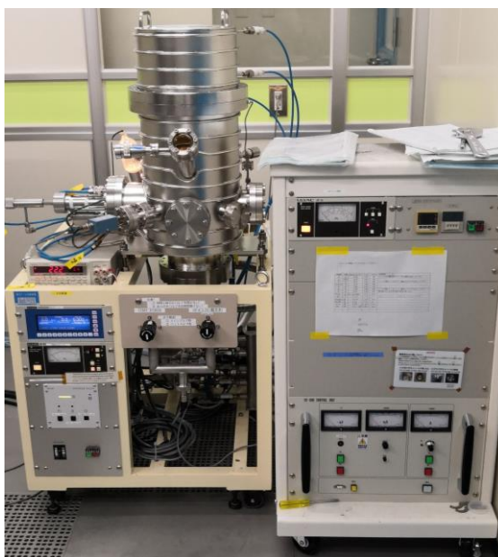
Figure 2.6 Photograph of Electron Beam Evaporation system.
