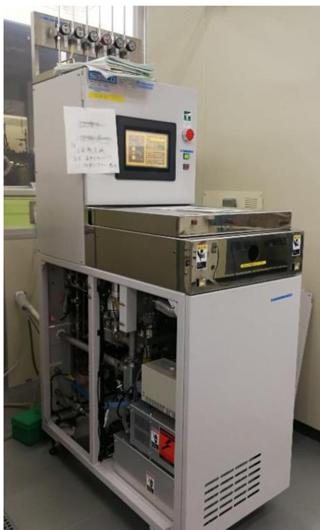
Figure 2.5 Photograph of Reactive Ion Etching system.
