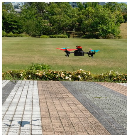
Figure 6: ArDrone 2.0 with GPS used for outdoor experiments.
